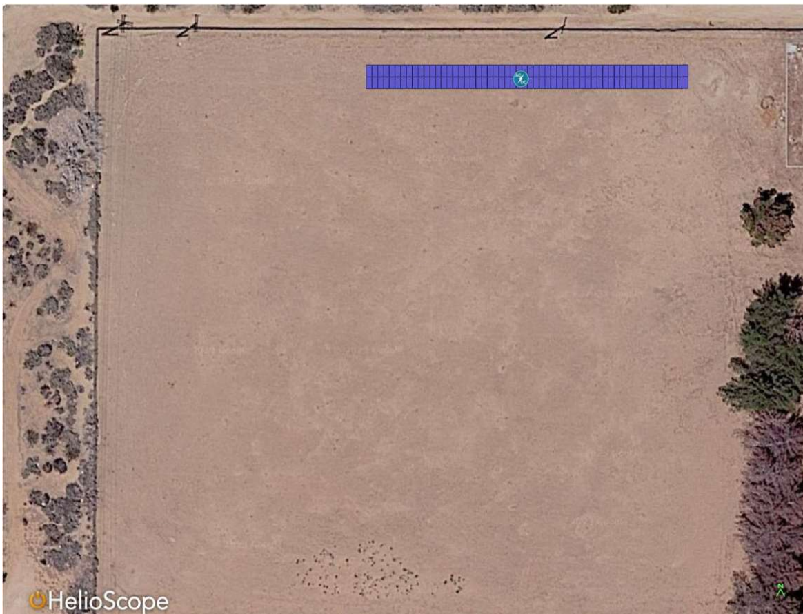
Figure 42:Popago Recommended Solar Array Layout
